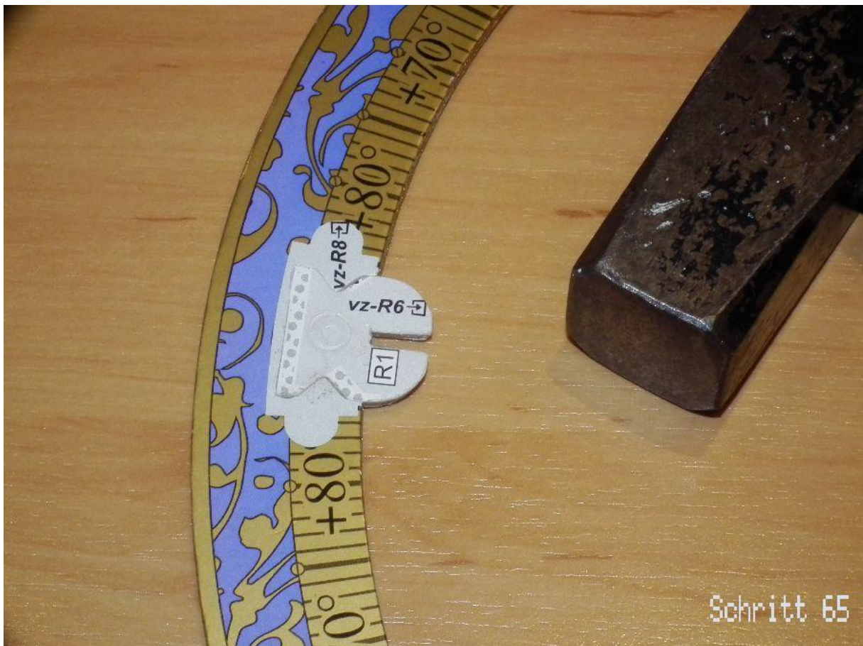
Step 65: A hammer is helpful when inserting the inner holders into the meridian to get an absolutely flat result.
