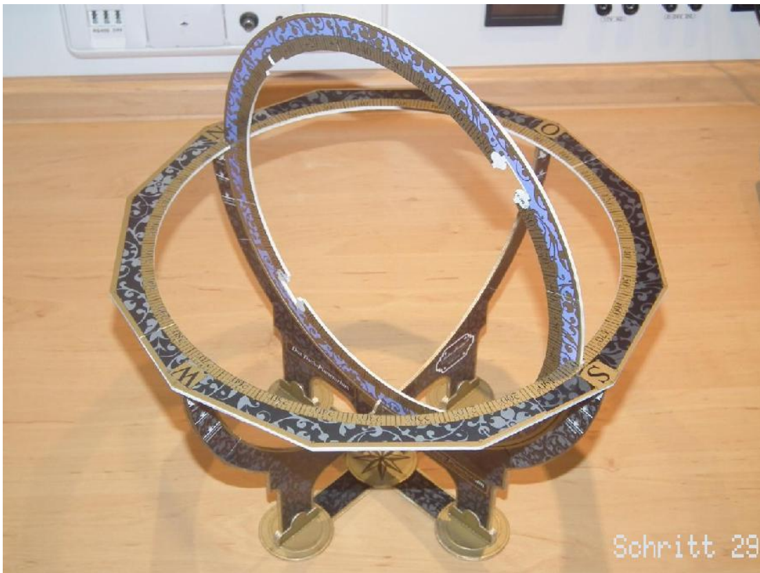
Step 29: Trying on the meridian in the horizon on the stand - it must be possible to turn the meridian without much resistance.
