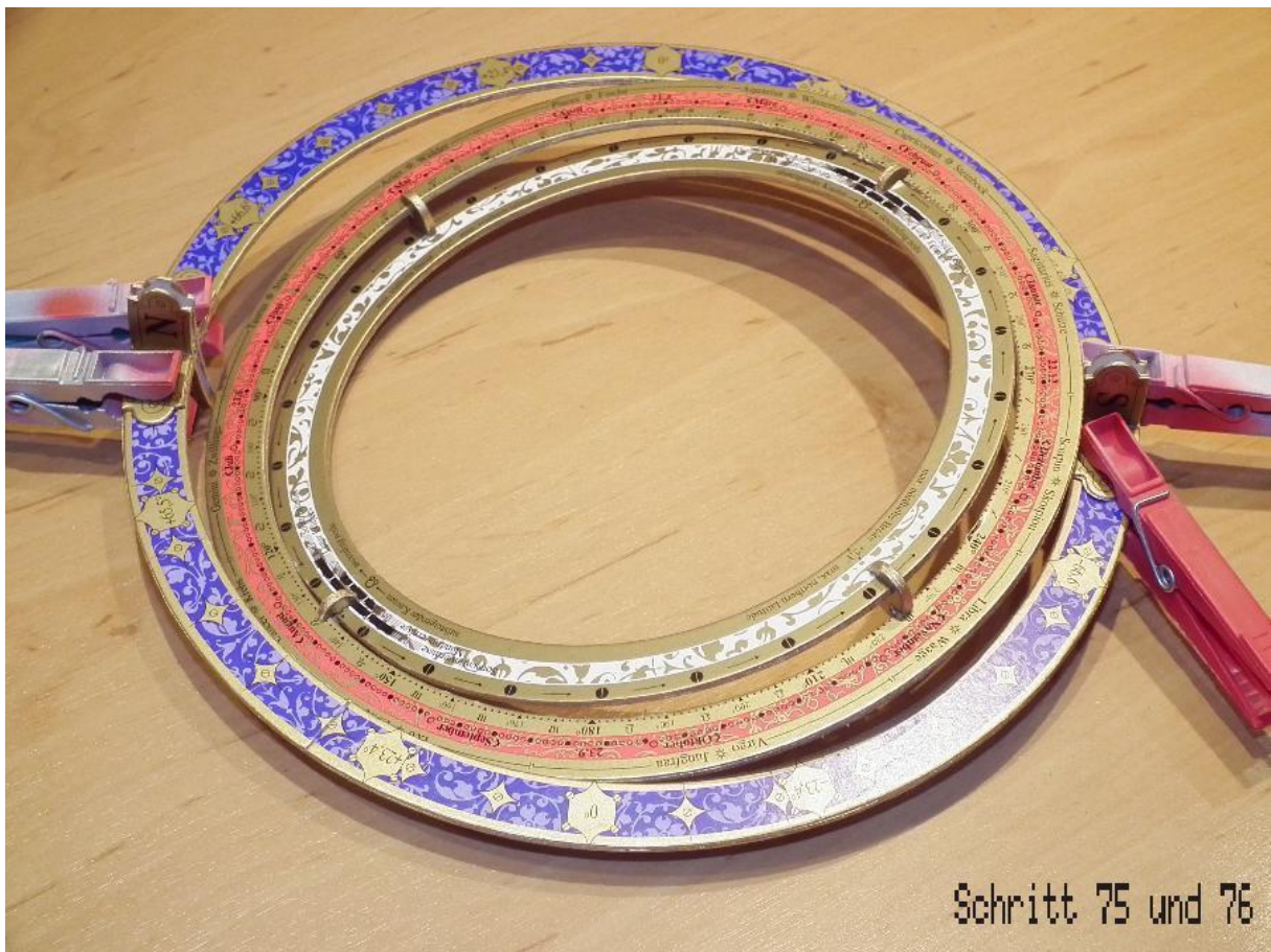
Steps 75 & 76: Before mounting the other arches, the ecliptic with the moon's orbit is installed.
