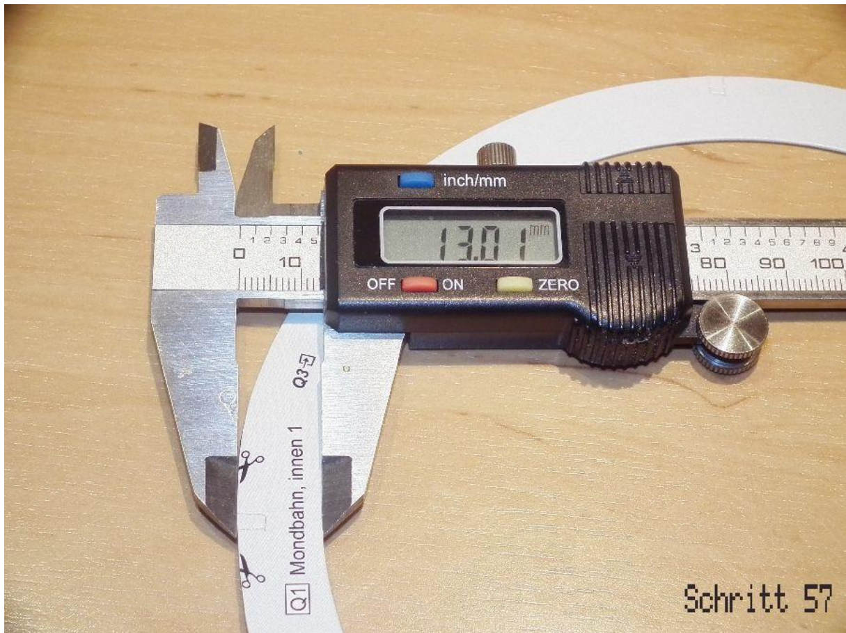
Step 57: The rings must not be wider than 13 mm at the points to be trimmed - recommendation: 12.5 mm.
