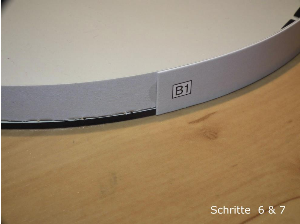
Steps 6 & 7: The picture shows that the second layer is glued onto the first layer and the edge of the mirror.
