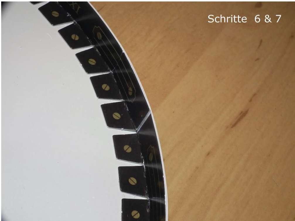
Steps 6 & 7: Glue the parts of the second layer overlapping on the first layer.
